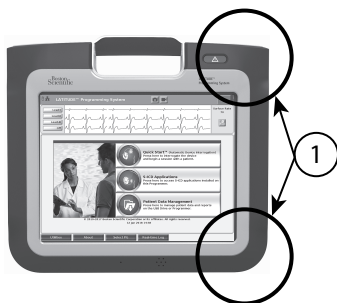
Figure 8. Front View of LATITUDE Programming System Indicating Approximate Antenna Locations Within the Enclosure
