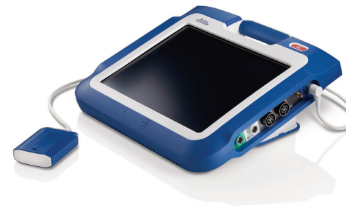
Doctors and nurses use a programmer to check an ICD and to communicate with it.
