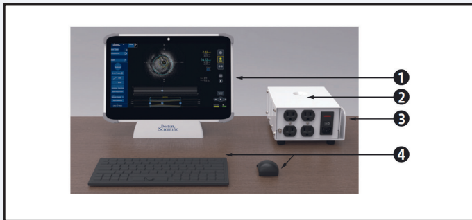
1 Tablet in Desktop Docking Station, 2 System Identification Label, 3 Isolation Station power button, 4 Keyboard and Mouse are installed in the control room adjacent to the procedure room.
