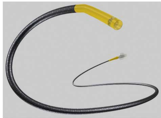
Fig. 1 Drawing to illustrate the unique design of the Direxion (Boston Scientific Corp.) microcatheter. The slotted nitinol design allows for excellent torqueability of the catheter shaft while retaining a similar pushability, trackability, and flexibility compared with other microcatheters. This results in precise steerability in combination with an angled-tip shape
