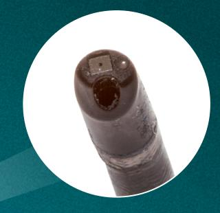
A 7.7F tip diameter and 9.5F [≤3.23mm] outer diameter easily fits the average human ureter with renal colic.9
